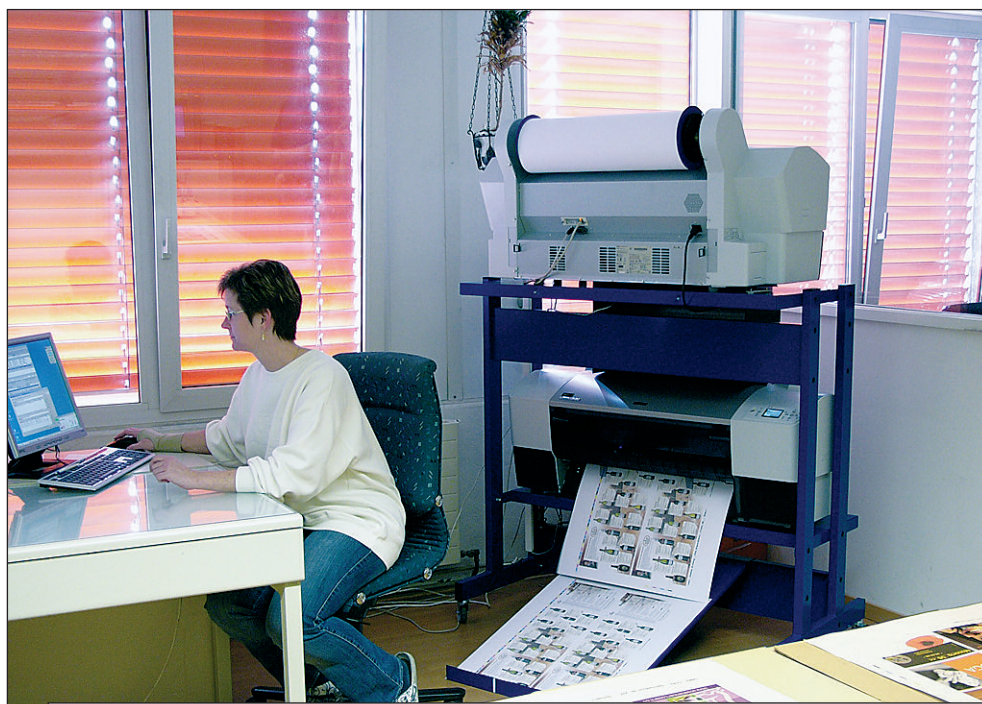
Preproofer 740 runs at up to 16 double-sided printed formproofs per hour.
